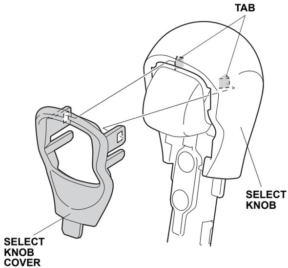
4. Remove the two screws from the select knob. Remove the select knob by pulling it up.
