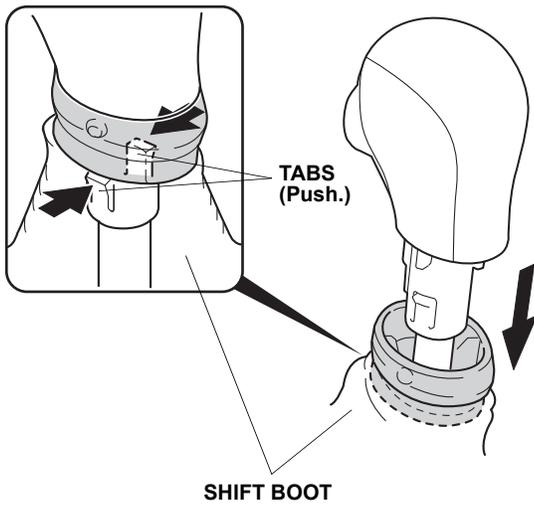
3. Pry on the bottom of the select knob cover and remove the cover.
