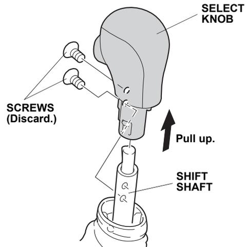
5. Install the new select knob with new screws. Using a torque screwdriver, torque the screws to 1.57 N·m (1.2 lbf-ft). Do not overtighten the screws.
